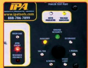
LED Showing an Open Circuit
